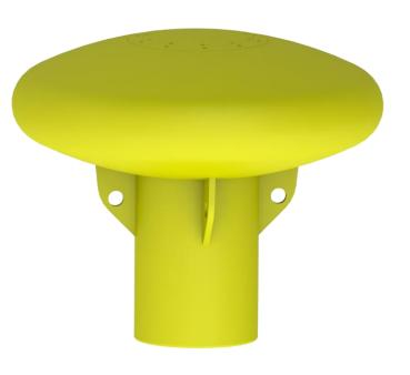
The Wave Guardian D1000SMN is a mini-oceanographic device for offshore monitoring, and can be adapted to perform water quality monitoring. Readings can be taken either dependent or independently and the probe will function correctly in fresh, salt or brackish water.
